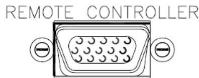
Fig 2-8 3305G Remote controller Connection
