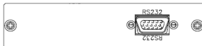
Fig 2-4 3300F RS232 Connection
