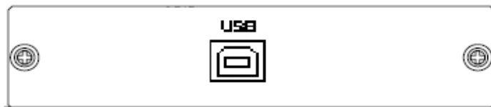
Fig 2-6 3300F USB Connection
