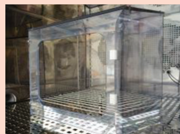
DIN 50017 – Condensation water test atmospheres
