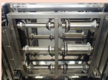
Cables/Wires winding accessory for 'Cold bend' testing
